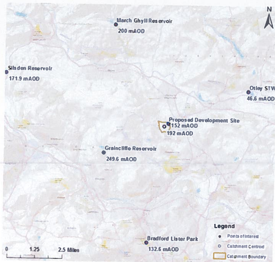
Figure 1: Raingauge and proposed development location with respective elevations. Catchment boundary with average elevation is also shown
